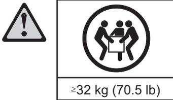
**Caution:** The weight of this part or unit is between 32 and 55 kg (70.5 and 121.2 lb). It takes three persons to safely lift this part or unit. (C010)
