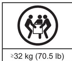
**Caution: The weight of this part or unit is between 32 and 55 kg (70.5 and 121.2 lb). It takes three persons to safely lift this part or unit. (C010)**
